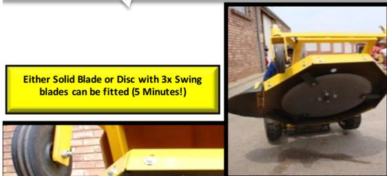
Either Solid Blade or Disc with 3x Swing blades can be fitted (5 Minutes!)
