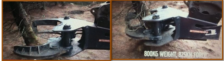
Tigerskid 100: Tractor mounted extraction grab for logs etc --Grab is . 33 cu meter
