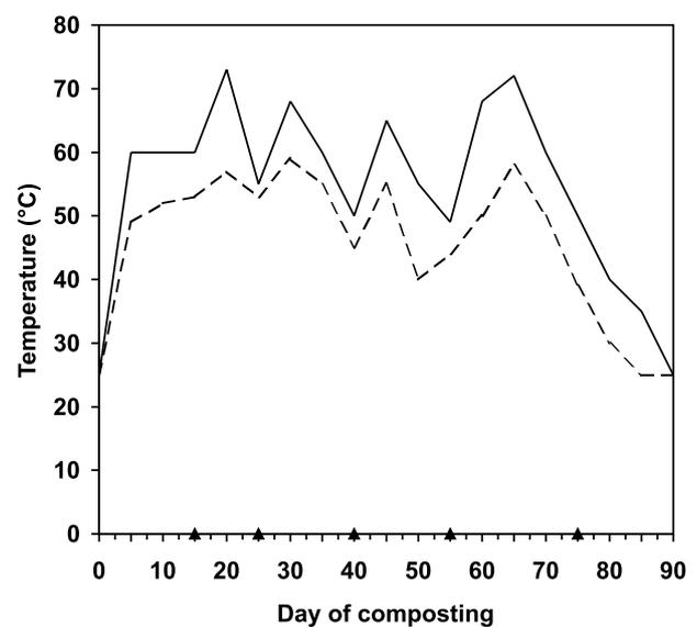
Fig. 1. Temperature fluctuations during composting of citrus waste: (---) 5 cm within pile; (—) 30 cm within pile; (▲) turning-over of pile (each value is the mean of four recordings).
