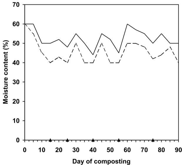
Fig. 2. Changes in moisture content of citrus waste during composting: (---) 5 cm within pile; (—) 30 cm within pile; (▲) turning-over of pile (each value is the mean of four samples).
