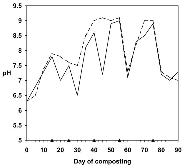
Fig. 3. Changes in pH of citrus waste during composting: (---) 5 cm within pile; (—) 30 cm within pile; (▲) turning-over of pile (each value is the mean of four samples).
