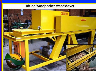
Ritlee 750. Cut 750mm -- Solid Blade or Disc + 3 Swing Blades. Height: Fixable with quick spacers. Gears 5xF, 1xR + N
