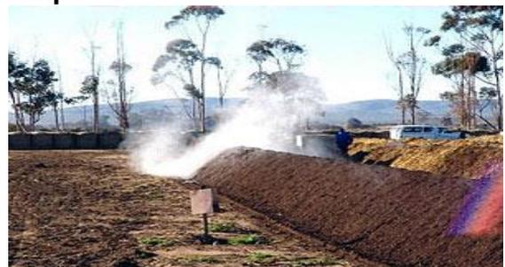
Turner thoroughly turns and mixes row at a speed which is most friendly to resident microbes, expels high temperatures, expels CO<sub>2</sub>, breaks up anaerobic clusters, mixes moisture, replaces expelled gasses with fresh air (Oxygen) and fluffs compost to allow easier flow of fresh air through row.
